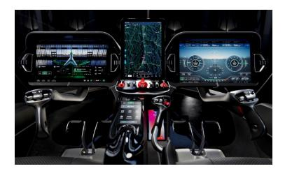
GL Studio provides an advanced toolset that has equipped Hill Helicopters to build an elegant user experience for the Visual Flight Rules (VFR) helicopter. The software is being leveraged to develop a certifiable software stack which is tested using piloted trials on an engineering simulator. The solution has enabled Hill Helicopters to link third-party systems such as the radio, intercom, GPS, and transponder with the User Interface application.
