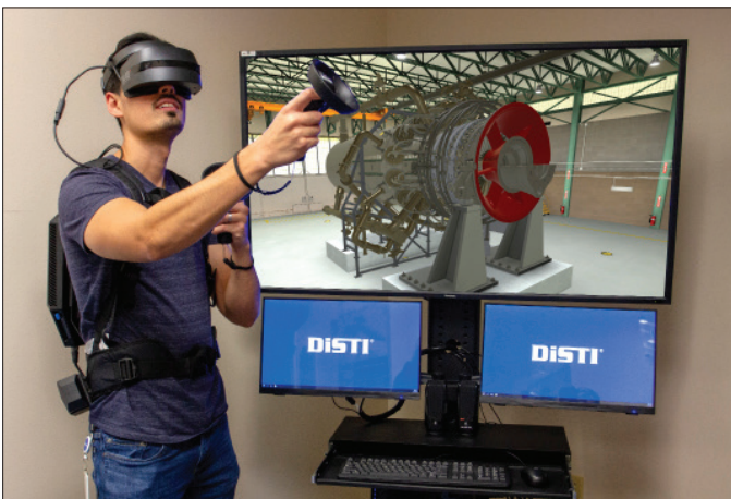
SGT-8000H VR prototype using HP's Z-Backpack for mobile VR training
