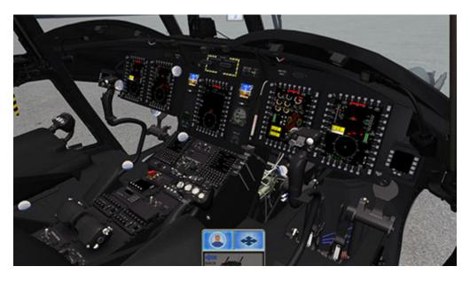
The CH-47F pre-built virtual cockpit is a fully interactive 3D repeater cockpit with zoom in and out capabilities for detailed instrumentation views and MFD displays with active buttons. Warnings Cautions and Advisory (WCA), Engine Instrument/Power Train page, Vertical Situation Display (VSD), Horizontal Situation Display (HSD), and the Fuel page are completely functional for each MFD.
