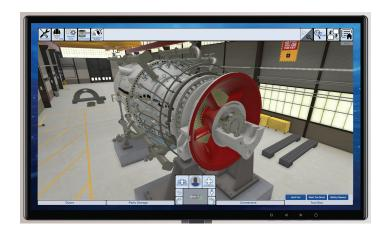
In this application, a technician uses Virtual Reality to be completely immersed in the virtual SGT6-4000F turbine and is required to identify potential damage to components inside of the gas turbine. This training is able to provide immediate feedback to the technician and assess performance to aid the technician in becoming more proficient in identifying damage and taking the subsequent corrective action.
