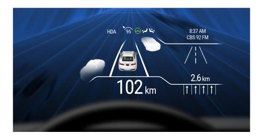
These redesigned automobiles will feature a 12-inch HUD that connects with the GPS data providing information like driving routes, driving assistance, and traffic signs. After activating the vehicle's advanced driver-assistance system (ADAS), the HUD can also offer traffic data of cars driving around the vehicle.
