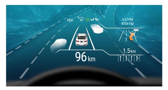
Built by Hyundai Mobis utilizing GL Studio<sup>®</sup> HMI software tools, the 12-inch HUD connects with the GPS data providing information like driving routes, driving assistance, and traffic signs. Upon activation of the vehicle's advanced driver-assistance system (ADAS), the HUD also offers traffic data of cars driving around the vehicle.
